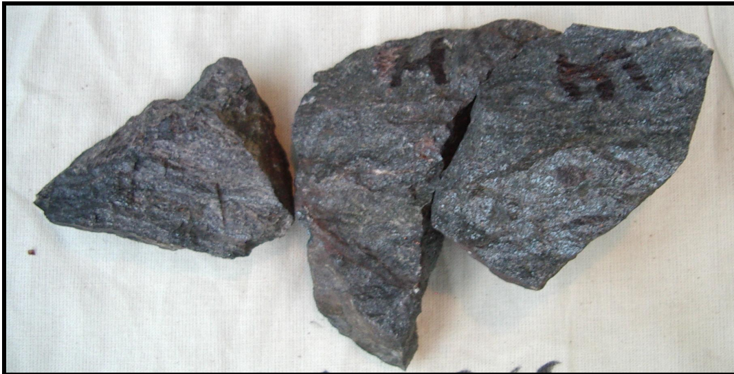
Selection of uranium ore types from waste dumps averaging 0.30% U 3 O 8
