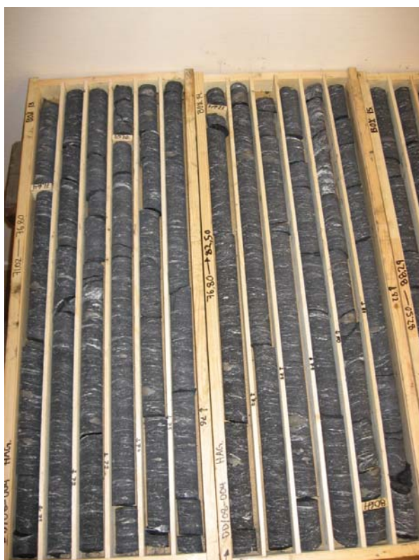
Example of Alum Shale from Hole DDHG-004 – this is 12m of a total 152m intercept.
