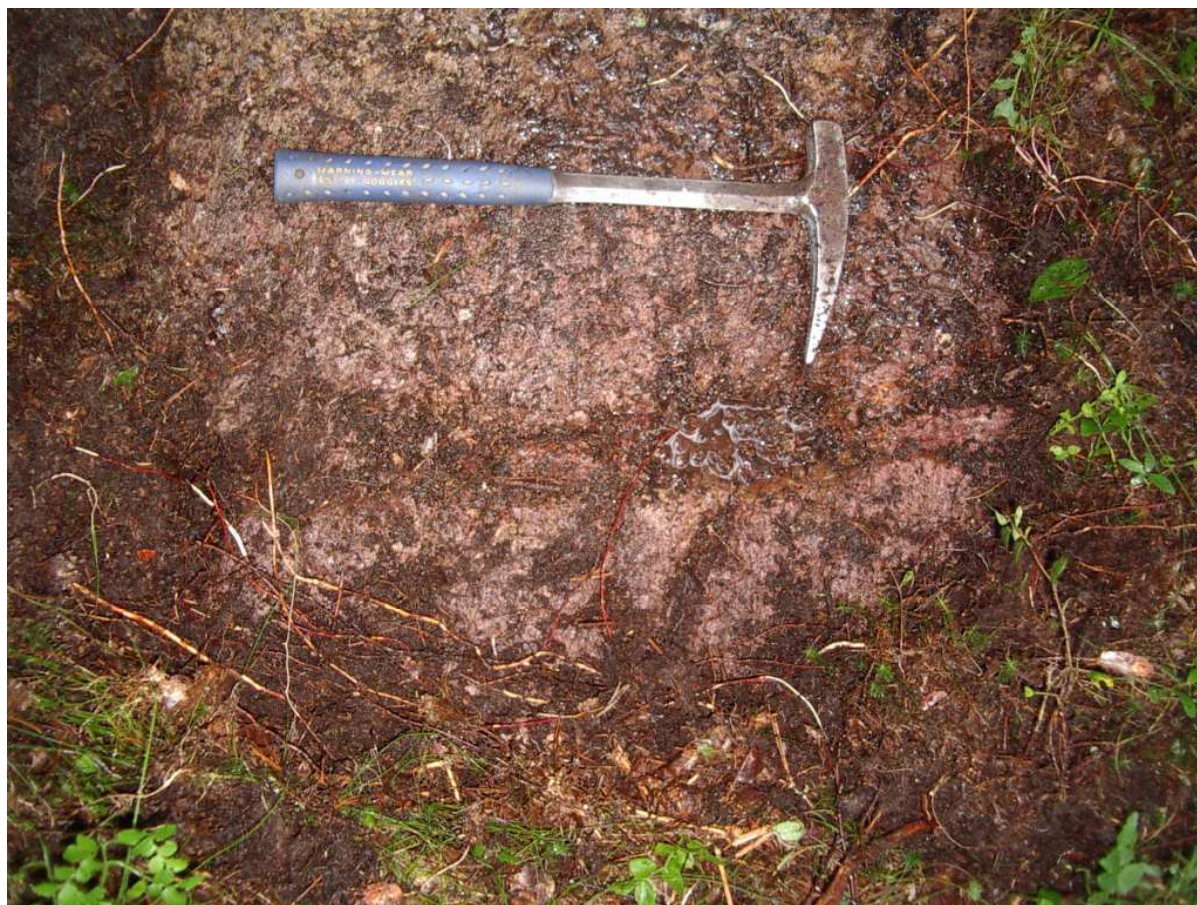
Silica hematite altered metasediment hosting uranium silver mineralisation in veins and veinlets at T ppetj rnet.
