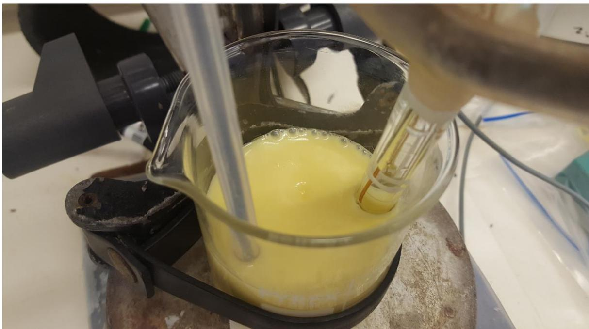
**Figure 2: UO<sub>4</sub> Yellowcake precipitation test**
